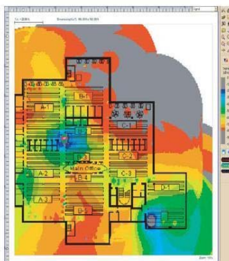
AirMagnet Survey Signal Analysis
